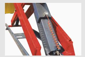
· Mechanical lock and air-driven safety release.
